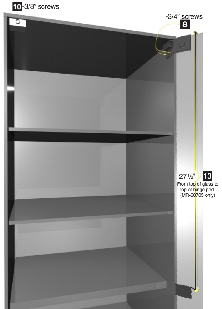
Figure 1. Door hardware installation.
